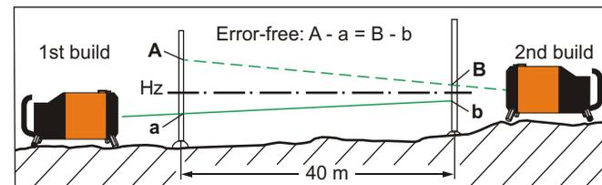
Although the laser is adjusted precisely by the manufacturer, jolts and strong vibrations can lead to maladjustment. The laser should therefore be checked before use:
